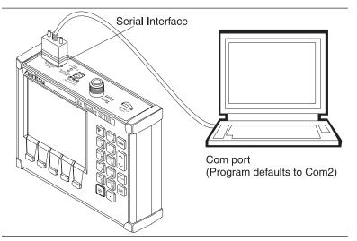
Figure 3-3. Equipment Setup for Site Master Tools Operation
