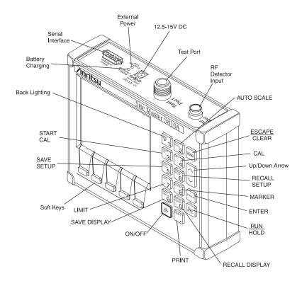
Figure 2-1. Site Master Controls and Connectors
