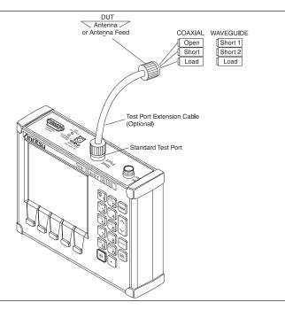
Figure 2-8. One-Port Measurement/Calibration Test Setup
