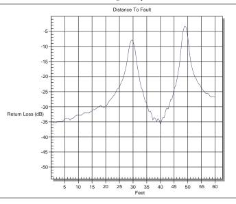
Figure 2-7. Minimum Side Lobe Windowing Example
