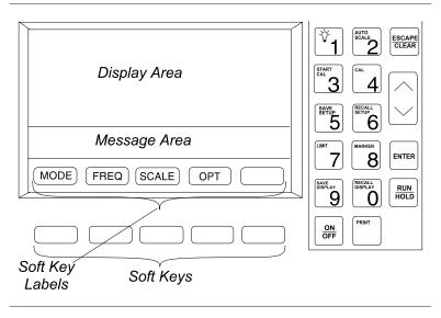
Figure 2-2. Site Master Front Panel Display Layout
