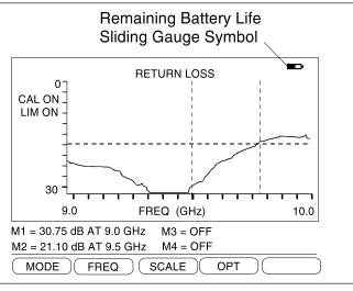
Figure 2-9. Battery Monitor
