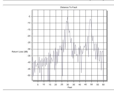
Figure 2-4. Rectangular Windowing Example
